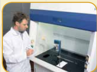
Face Velocity Measurement Test
