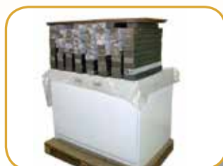
Actual photo during Cabinet Load Testing
