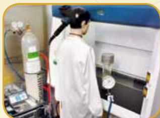
Tracer Gas (SF 6 ) Containment Test
