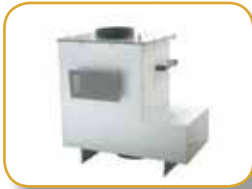
Image 1: Top section of scrubber placed on top of the fume hood. There is an acrylic viewing panel, a packed bed, a liquid spray section as well as a demister in this unit.
