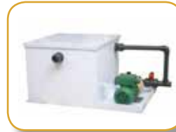
Image 2: Bottom section of scrubber placed inside the base cabinet. Consists of a reservoir for scrubbing liquor and a pump which recirculates the liquor back into the system.
